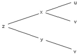
$$\frac{\partial z}{\partial u} = \frac{\partial z}{\partial x} \frac{\partial x}{\partial u} = 2xy^2 \cdot v = 2uv \cdot v^4 \cdot v = 2uv^6$$
